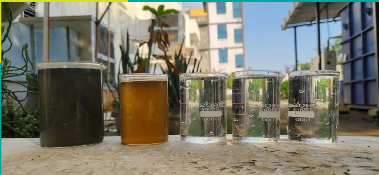
✓ Coloured wastewater (extreme left) from textile facility in Noida, India (garment washing) and treated water (extreme right) using Indra Electro module (3 m 3 /hour) for process reuse
